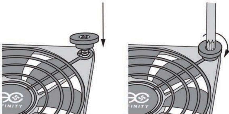
Insert the rubber feet through the guard and onto the fan's screwhole. Turn until you feel the screw tightening but do not overextend or the screw will slip through the rubber feet. Depending on your setup, you may not need a rubber feet on every hole, please see pages 10 to 12.
