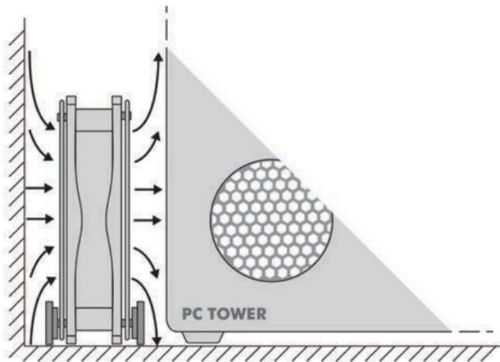
The Multipurpose Fan can also stand upright to help circulate air in narrow places such as inside a computer desk or home theater cabinet. The fan helps push hot air out, allowing colder air to come in. You would need to install four rubber feet on the fan's bottom.
