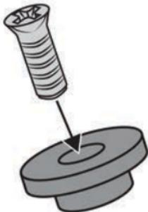
Place the screw inside the hole located at the rubber foot's base. Push the screw's head until its thread shows up on the other end.
