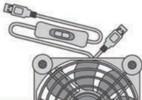
Each fan unit includes an USB port that can connect to an another fan. Up to four fans can be powered through one dedicated USB port or outlet source.
