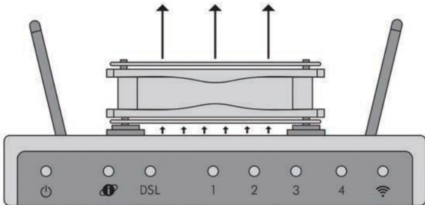
The Multipurpose Fan can be placed above electronics that have vents on the top, such as a modem box or gaming station, to help draw out hot air. You would need to install four rubber feet on the fan's base.
