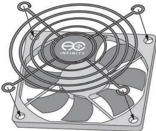
Position the front guard on top of the fan's frontal frame, aligning each of the four screw holes. To locate the front of the fan, find the side that contains plastic beams.
