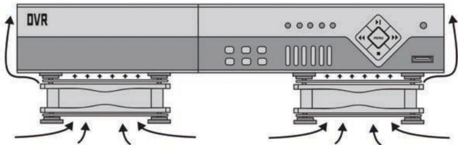
The Multipurpose Fan can also be placed below electronics to help accelerate the rising hot air. Up to four units can be daisy chained together to create a base for larger electronics, see page 13. Eight rubber feet are required for each fan.
