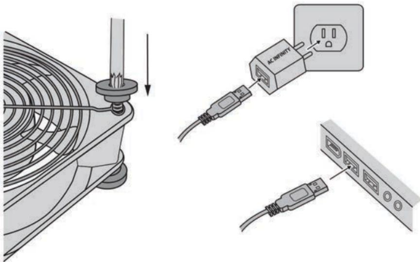
Repeat to secure the back guard onto the backside of the fan. Please make sure the elevated side of the guard is facing outwards or it will come into contact with the fan's impeller. To power the fan, plug it into a USB port or using the power adapter, plug it into an outlet.
